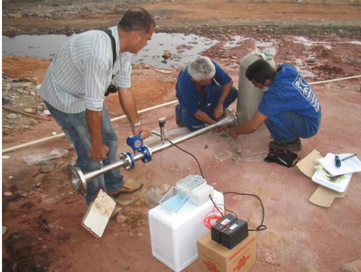
Figure 3. Measurement of the outflow of a well of biogas
