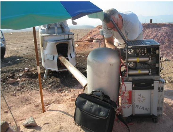
Figure 2. Monitoring of biogas using the portable chromatograph.
